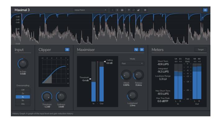
Maximal 3 is a loudness maximiser offering true-peak brickwall limiting, variable shape soft-clipping, and substantial loudness metering options, perfect for mixing and mastering.
