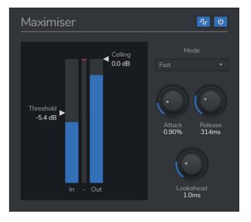
You can hold the CTRL/CMD key to link the two sliders, so that adjusting the level of one affects the other by the same amount. This lets you use the maximiser as limiter, adjusting the threshold without affecting the overall level.
