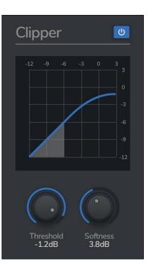
The clipper also has an advantage when it comes before limiting - if you use it to shave of the highest peaks in the audio, the limiter doesn't have to work as hard.
